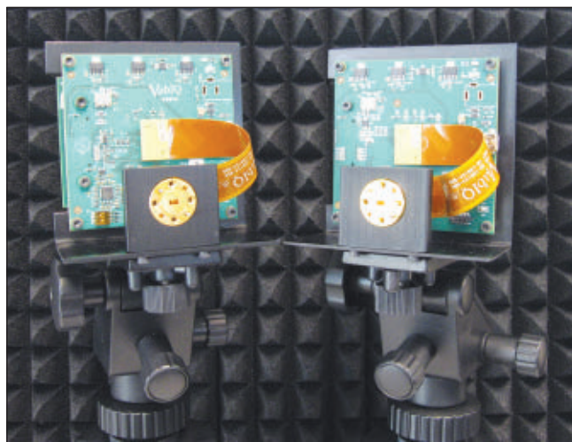
▲ Fig. 1 The PEM003-KIT's primary components are the transmitter and receiver PC boards, shown mounted on their tripods, and WR15 waveguide antenna modules.
